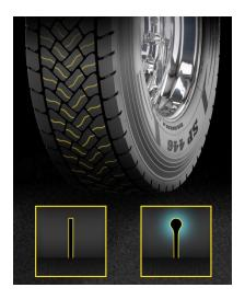
Raindrop shape sipe channel Sipes designed with sharp corners exhibit concentrated stress levels due to block movement in service -> M+S and 3PMSF marking, sipes are robust against all service conditions
