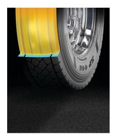
Dual layer tread compound The tread features a top layer highly resistant against abrasion, a low-hysteresis bottom layer that minimizes rolling resistance. -> 10% higher mileage\*, low rolling resistance
